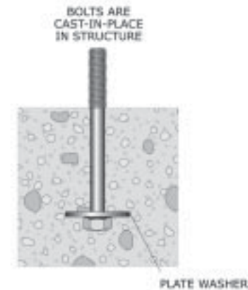
Figure 136: Bolting equipment to cast-in-place anchors.
