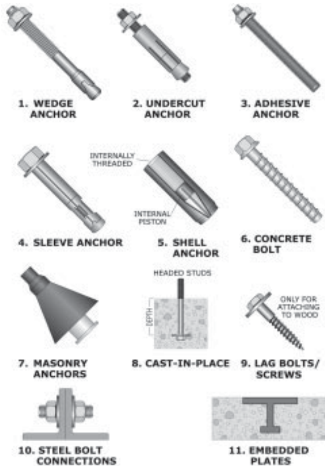
Figure 127: Types of anchors.
