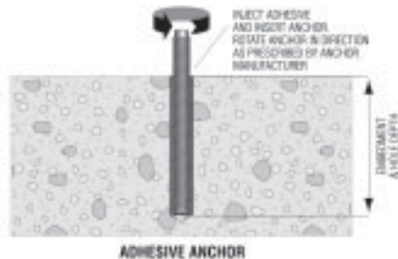
Figure 131: Adhesive anchor installation.
